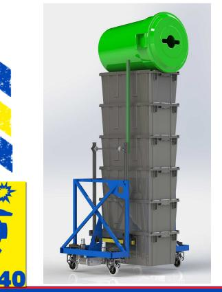
DB 11 was largely designed around the stack of totes it needed to build and transport to score.
