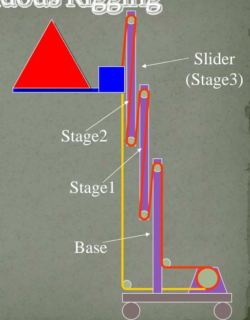
Extension: Continuous Internal Rigging
