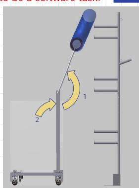
2) Elbow & Shoulder deploy to achieve scoring height. Ubertube is naturally at a good orientation for scoring
