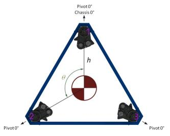
center-point and the pivot axes and an angle  $\theta$ = 120° (2 $\pi$ /3R) between each pivot axis around the chassis center-point. Swerve modules are mounted so that each module's 0° calibration axis faces directly away from the chassis center-point. Swerve modules are identified by numbers 1, 2 & 3 following right-hand rule.
