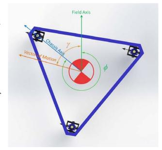
The joystick steering direction,  $\gamma(^{\circ})$ , is now relative to the field axis, not the chassis axis.
