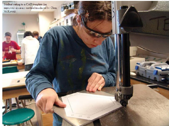
Cutting a from a CAD template (an improved-accuracy method created by Clem McKown)
