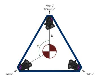
center-point and the pivot axes and an angle  $\theta$ = 120° (2 $\pi$ /3R) between each pivot axis around the chassis center-point. Swerve modules are mounted so that each module's 0° calibration axis faces directly away from the chassis center-point. Swerve modules are identified by numbers 1, 2 & 3 following right-hand rule.
