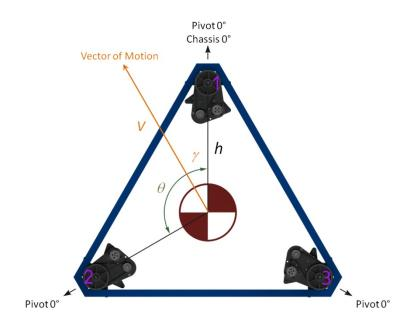
In *Crab Mode*, the primary joystick applies a *Vector of Motion* to the chassis described in the previous section. This *Vector of Motion* provides both angular direction  $(\gamma)$  and power/speed (V) information.
