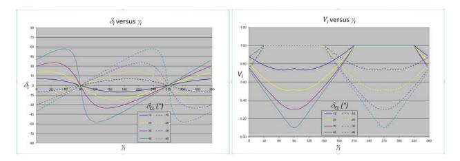
When  $\delta_{CL}$  is negated, the affect on both  $\delta_i$  and  $V_i$  is a phase shift in  $\gamma_i$  of 180°. So, a look-up table having only positive (or only negative)  $\delta_{CL}$ 's can be used to cover the entire turning range, but for negative  $\delta_{CL}$ 's, the  $\gamma_i$  look-up would need to be shifted by 180° (and checked for 0-360° range).
