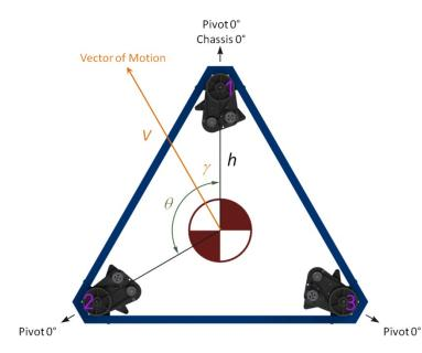
In *Crab Mode*, the primary joystick applies a *Vector of Motion* to the chassis described in the previous section. This *Vector of Motion* provides both angular direction  $(\gamma)$  and power/speed (V) information.
