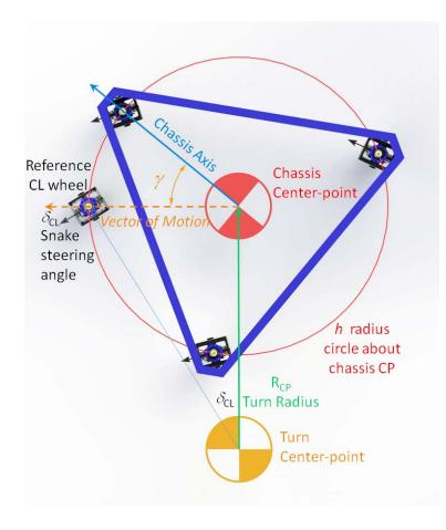
In the 2009 swerve white papers, I introduced the concept of a "reference CL wheel", a useful tool for working through the mathematics around Snake Mode. The "reference CL wheel" concept will be employed again here.
