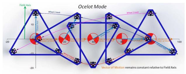
Angle between Chassis Axis and Vector of Motion changes To maintain constant Vector of Motion through a "turn" (for constant joystick input)
