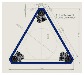
A dimensioned schematic of such a chassis is provided in Figure 1.
